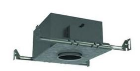
**BODY FINISH** Galvanized Steel WATTAGE 20W DIMMER Low Voltage Magnetic DIMENSIONS 15.5"L x 10"W x 7.1"H **BULB NOT INCLUDED** LAMP 1 x MR16/Bipin/20W/120V Halogen 1 x MR16/GU5.3 (bipin)/12V LED Technical Information CEILING TYPE Drywall with Trim HOUSING TYPE Chicago plenum approved HOUSING HEIGHT APERTURE SIZE 3.000"
