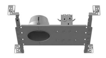
TRIM COLOR N/A **BODY FINISH** Galvanized Steel WATTAGE /2\M DIMMER Low Voltage Electronic DIMENSIONS 12"L x 7.5"W x 3.5"H **BULB NOT INCLUDED** LAMP MR16/GU5.3 (bipin)/42W/12V Halogen 1 x MR16/GU5.3 (bipin)/12V LED Technical Information CEILING TYPE Drywall with Trim HOUSING TYPE New Construction NON IC HOUSING HEIGHT APERTURE SIZE 4.000" SPEC # CLT106641
