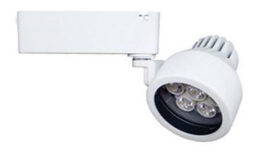
SHADE COLOR N/A BODY FINISH White WATTAGE 18\\/ DIMMER Dimmable DIMENSIONS 5.9"W x 4.4"H x 3.7"D INTEGRATED LED MODULE LAMP 1 x LED/18W/120V LED Technical Information LUMINOUS FLUX 1200 lumens LUMENS/WATT 66.67 LAMP COLOR 2700K COLOR RENDERING 80 CRI BEAM ANGLE 25° SPEC # CNT109538
