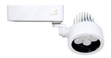
**BODY FINISH** White WATTAGE 27\// DIMMER Dimmable DIMENSIONS 5.9"W x 4.4"H x 3.9"D INTEGRATED LED MODULE LAMP 1 x LED/27W/120V LED Technical Information LUMINOUS FLUX 1710 lumens LUMENS/WATT 63.33 COLOR RENDERING 80 CRI
