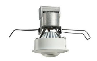
TRIM COLOR N/A BODY FINISH White WATTAGE 5\// DIMMER Dimmable DIMENSIONS 2.62"W x 3.25"H INTEGRATED LED MODULE LAMP 1 x LED/5W/12V LED Technical Information LAMP COLOR 2700K BEAM ANGLE SPEC # JUN111274
