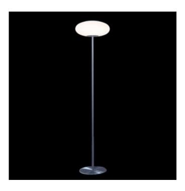
SHADE COLOR Satin White BODY FINISH Satin Nickel WATTAGE 75\// DIMMER Included DIMENSIONS 13.75"W x 59"H BULB INCLUDED LAMP 1 x T4/D.C. Bayonet (BA15D)/75W/120V Halogen Technical Information LUMINOUS FLUX 1100 lumens LUMENS/WATT 14.67 LAMP COLOR 2900K SPEC # HLK157357
