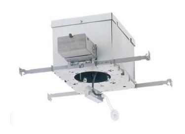
TRIM COLOR N/A BODY FINISH Galvanized Steel WATTAGE N/A DIMMER Dimmable DIMENSIONS 15.5"L x 9"W x 7.3"H **BULB NOT INCLUDED** LAMP 1 x MR16/GU5.3 (bipin)/12V Halogen 1 x MR16/GU5.3 (bipin)/12V LED Technical Information CEILING TYPE Drywall with Trim HOUSING TYPE New construction IC Airtight HOUSING HEIGHT PRODUCT DIMENSIONS 3.69 inch ceiling cutout SPEC # LTL19220
