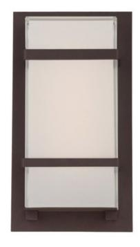
**BODY FINISH** Bronze WATTAGE 12W DIMMER Low Voltage Electronic DIMENSIONS 6"W x 11"H x 3"D INTEGRATED LED MODULE 1 x LED/12W/120V LED LAMP Technical Information LUMINOUS FLUX 327 lumens LUMENS/WATT 27.25 LAMP COLOR 3000K COLOR RENDERING 90 CRI
