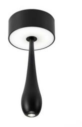
SHADE COLOR N/A **BODY FINISH** Black WATTAGE 9.5W DIMMER Not Dimmable 4.75"W x 10.4"H DIMENSIONS INTEGRATED LED MODULE 1 x LED/12V LED LAMP 1 x LED/12V LED Technical Information LUMINOUS FLUX 295 lumens LUMENS/WATT 49.17 **BEAM ANGLE** 56° SPEC #
