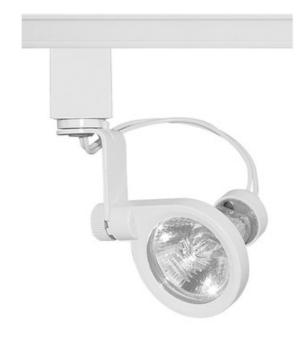
SHADE COLOR N/A BODY FINISH White WATTAGE 35W DIMMER Dimmable DIMENSIONS 3.75"L x 1.63"W x 1.63"D BULB NOT INCLUDED LAMP 1 x MR11/GU4/35W/12V Halogen
