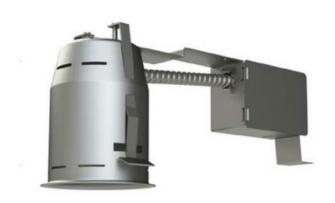
TRIM COLOR N/A **BODY FINISH** Galvanized Steel WATTAGE 2014/ DIMMER Low Voltage Electronic DIMENSIONS 12.1"L x 4.18"W x 6"H **BULB NOT INCLUDED** LAMP 1 x MR16/GU5.3 (bipin)/20W/12V Halogen 1 x MR16/GU5.3 (bipin)/12V LED Technical Information CEILING TYPE Drywall with Trim HOUSING TYPE Remodel NON IC HOUSING HEIGHT APERTURE SIZE 3.000" SPEC # CLT3806
