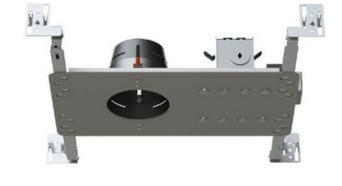
TRIM COLOR N/A BODY FINISH Galvanized Steel WATTAGE 50W DIMMER Low Voltage Magnetic DIMENSIONS 15.38"L x 10"W x 3.4"H **BULB NOT INCLUDED** LAMP 1 x MR16/GU5.3 (bipin)/50W/12V Halogen 1 x MR16/GU5.3 (bipin)/12V LED Technical Information CEILING TYPE Drywall with Trim HOUSING TYPE New Construction NON IC HOUSING HEIGHT APERTURE SIZE 3.500" SPEC # CLT3814
