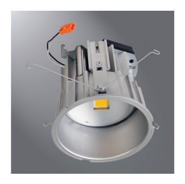
**BODY FINISH** N/A WATTAGE 13.8W DIMMER N/A DIMENSIONS 5.75"W x 6.19"H INTEGRATED LED MODULE LAMP 1 x LED/13.8W/120V LED Technical Information LAMP COLOR 3045K COLOR RENDERING 80 CRI LAMP LIFE 50000 hours CEILING TYPE Drywall with Trim
