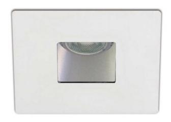
TRIM COLOR N/A **BODY FINISH** Matte White/ Anodized Reflector WATTAGE 50W DIMMER Dimmable DIMENSIONS 4.25"W x 2"H x 4.25"D **BULB NOT INCLUDED** LAMP 1 x MR16/GU5.3 (bipin)/50W/12V Halogen 1 x MR16/GU5.3 (bipin)/12V LED 1 x MR16/GU10/120V Halogen 1 x MR16/GU10/120V I ED 1 x PAR16/Medium (E26)/120V LED Technical Information **FUNCTION** Wall Washer CEILING TYPE Drywall with Trim APERTURE SHAPE Pinhole APERTURE SIZE 1.750" SPEC # CLT51556
