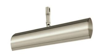
SHADE COLOR N/A BODY FINISH Satin Nickel WATTAGE 3/1 8\M DIMMER Dimmable DIMENSIONS 13.56"W x 3.07"H x 1.92"D INTEGRATED LED MODULE LAMP 1 x LED/34.8W/12V LED Technical Information LUMINOUS FLUX 782 lumens LUMENS/WATT 22.47 LAMP COLOR 2949K COLOR RENDERING 84 CRI SPEC # EDG56209
