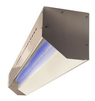
SHADE COLOR N/A BODY FINISH Aluminum WATTAGE 13\// DIMMER Dimmable DIMENSIONS 12"L x 5.6"H x 5.5"D INTEGRATED LED MODULE LAMP LED/13W/120V LED Technical Information LAMP LIFE 50000 hours
