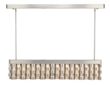
SHADE COLOR N/A BODY FINISH Satin Nickel WATTAGE 42.8W DIMMER Dimmable DIMENSIONS 1.75"W x 9.75"H x 46.4"D INTEGRATED LED MODULE LAMP 18 x LED/120V LED
