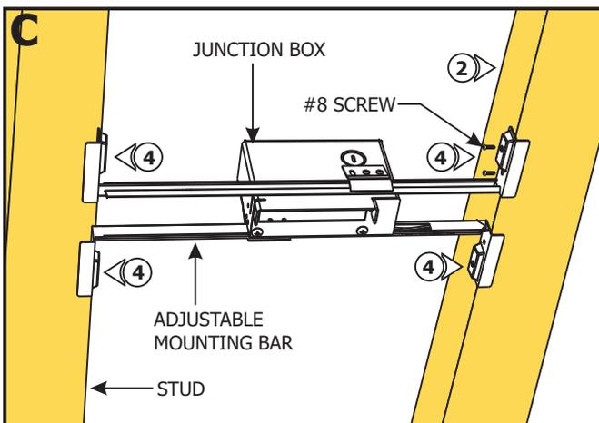
**NOTE:** The adjustable mounting bars mount to studs that are spaced 16" to 24" apart.
