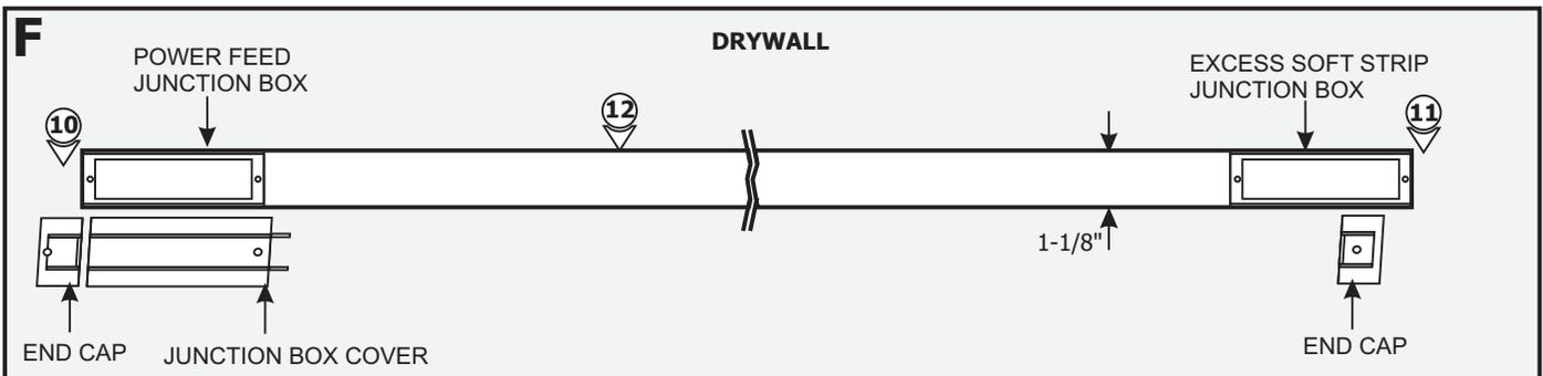
**10: For the Power Feed Junction Box:** Secure the end cap & junction box cover with the 4-40 screw, and make any reference marks that are needed.
