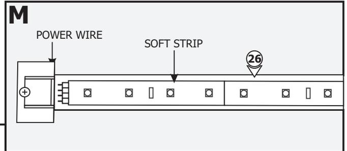
**26:** Push the soft strip male end onto the soft strip power wire.
