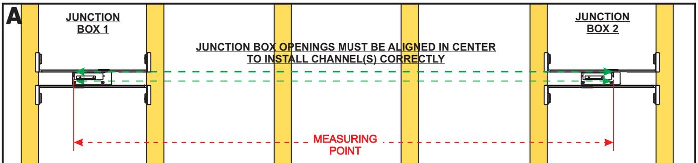
**NOTE:** Select the location between the two studs where the channel is going to be mounted. Each end of the channel must be into a junction box opening. One junction box is used as the power feed and the other one for excess soft strip.
