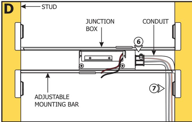
**5:** Remove a knockout to install the power line conduit.
