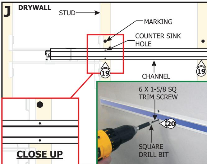
**19:** Using the mark locations on the drywall, carefully make a hole to each side of the channel using the square drill bit with counter sink provided.
