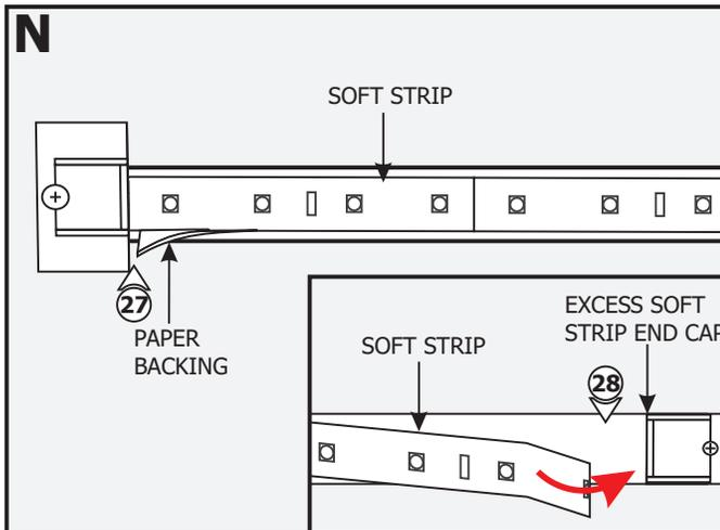
**27:** Carefully remove the backing from the LED soft strip, make sure not to remove the tape from the soft strip. Firmly press down the adhesive portion of the soft strip onto the channel surface while removing the rest of the backing, making sure there are no air bubbles that can cause surface irregularities.
