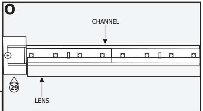
**29:** Remove the tape from the lens and snap lens into the channel.
