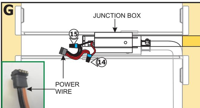
**14:** Connect the red power supply (24VDC+) wires to power wire red strip wire with a wire nut inside the electrical box.
