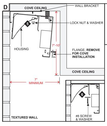
**NOTE:** For a cove (7"-10") installation, remove the flange for a tighter fit installation.
