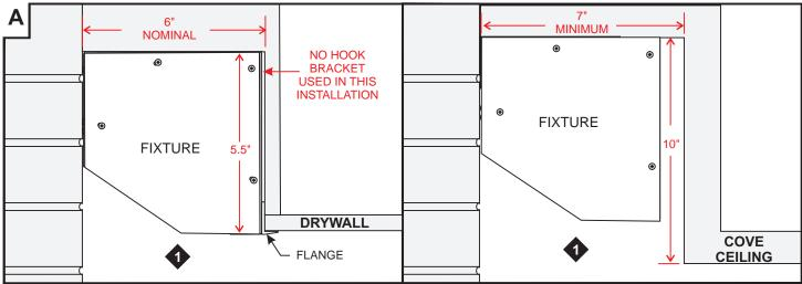
1: Determine the location where the fixture will be installed. In most cases fixture will be installed in either a flush ceiling or in a in-depth cove installation.
