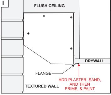
**NOTE:** If the fixture was installed against drywall, plaster, sand, and then prime & paint the flange to complete the installation.
