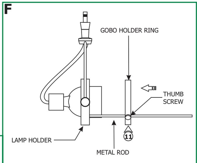
**11:** Place the gobo holder ring holes onto the metal rods. Slide the gobo holder ring back against the snoot and tighten the thumb screws.
