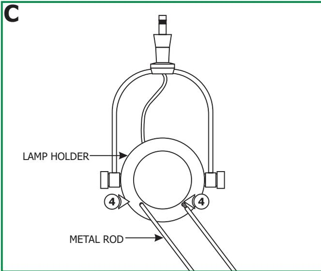
**4:** Screw the two metal rods completely into the threaded holes on the lamp holder of the Harley fixture.
