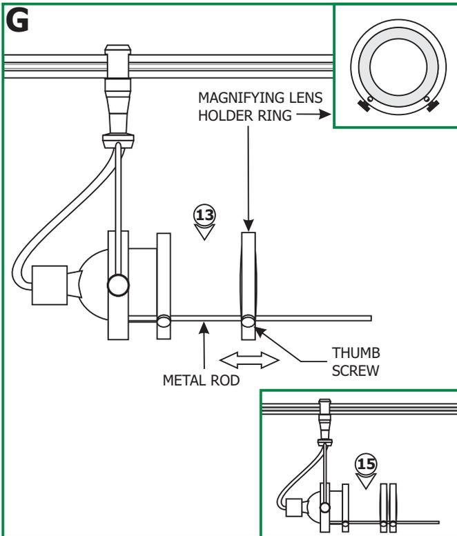
**NOTE:** The projected gobo image on the wall gets larger and the intensity of the image gets dimmer as the fixture is installed farther from the wall.
