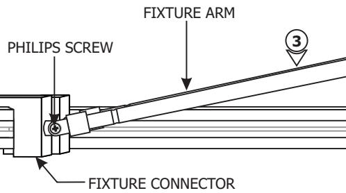
**3:** Rotate the fixture arms to the desired position. If necessary tighten the Phillips screws on the fixture connector to hold the fixture in place.
