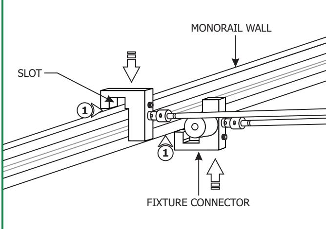
**1:** Place one fixture connector slot from the top and the other one from the bottom onto the Monorail Wall.
