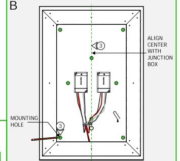
3: Align the mounting plate hole with the power line conduit, or junction box. Use the mounting plate as a template to mark eight mounting holes (highlighted in GREEN) onto the wall.
