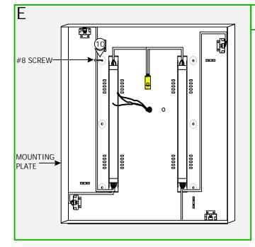
10: Level the mounting bracket horizontally and use the #8 screws to secure the mounting plate to the anchors.
