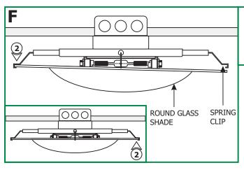
2: Place the edge of the round glass shade into two adjacent spring clips. Slightly push the glass shade against these two spring clips and simultaneously slide the other edge into the other two spring clips. Make sure that the round glass shade sits properly into the four spring clips.
