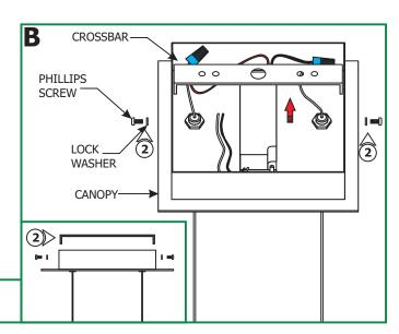
**2:** Remove the two Phillip screws and lock washers on the sides of the canopy, and carefully pull the crossbar out.
