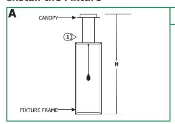
**1:** Determine the desired fixture height **(H)**, from the bottom of the fixture frame to the top the canopy.
