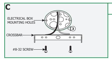
**3:** Mount the crossbar to the electrical box holes with the provided #8-32 screws.
