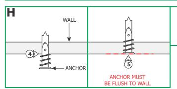
4: Tap the anchors onto the marked points up to the threaded portion with a hammer.
