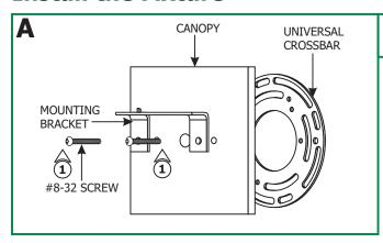
2: Mount the universal crossbar to the electrical box holes with the provided #8-32 screws so that the two inner threaded holes (spaced 2-1/8" apart) on crossbar are leveled horizontally.
