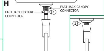
**1:** Use fingers to tighten the Fast Jack fixture connector into the Fast Jack canopy connector.
