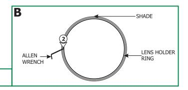
**2:** Use a small Allen wrench or a pen point to loosen and remove the lens holder ring from the shade.
