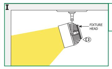
**2:** Rotate the fixture head to properly accent desired location.
