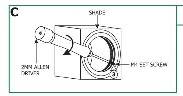
**3:** Tighten the M4 set screw on the front of the shade with the 2mm Allen driver provided.
