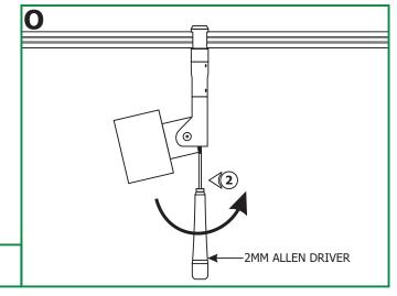
**2:** Use the 2mm Allen driver on the bottom of the Box arm to tilt the head up or down.
