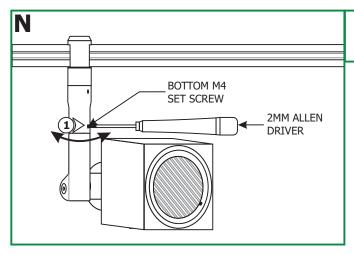
1: Rotate the fixture to the desired position and lock it in place by tightening the bottom M4 set screw with the 2mm Allen driver.
