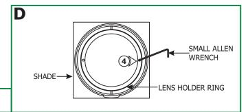
**4:** From the inside of the shade, use a small Allen wrench or a pen point to loosen and remove the lens holder ring.
