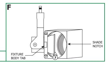
7: Line up the notch on the shade with the tabs on the fixture body and push it completely until it snaps in place properly.
