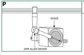
**3:** Place the 2mm Allen driver into the M4 set screw on the front of the shade to rotate the lens to the desired position. Tighten the M4 set screw to lock the lens in position.
