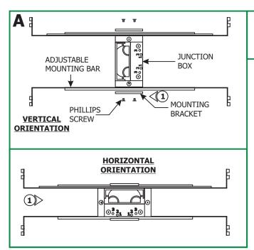
**1:** Mount each adjustable mounting bar to one side of the junction box (mounts to any side of the housing depending on the orientation of the channel) and secure them with the mounting brackets and two Phillips screws provided.
