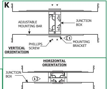
1: Mount each adjustable mounting bar to one side of the junction box (mounts to any side of the housing depending on the orientation of the channel) and secure them with the mounting brackets and two Phillips screws provided.
