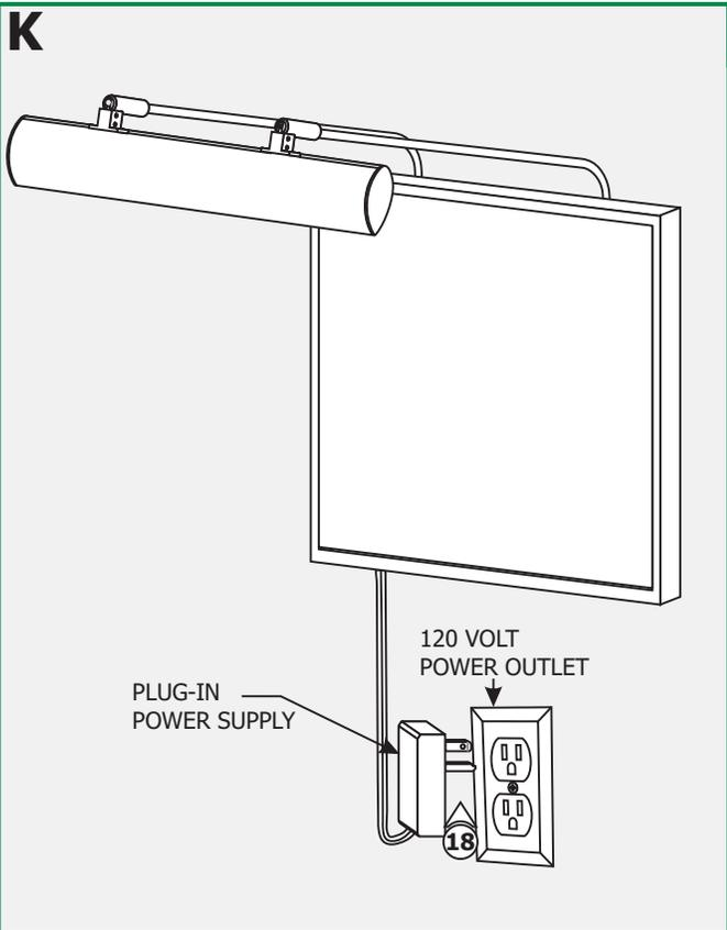
**18:** Plug the power supply into the 120 volt power outlet.
