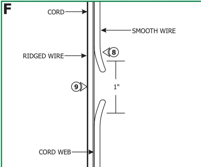
**8:** Select the location on the cord where the switch will be installed.
