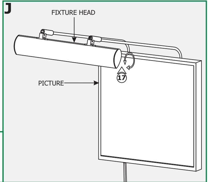
**17:** Rotate the fixture head to properly wash the picture with light.
