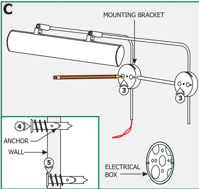
**NOTE:** The Cody 12" canopy mount must be installed right above the electrical box.
