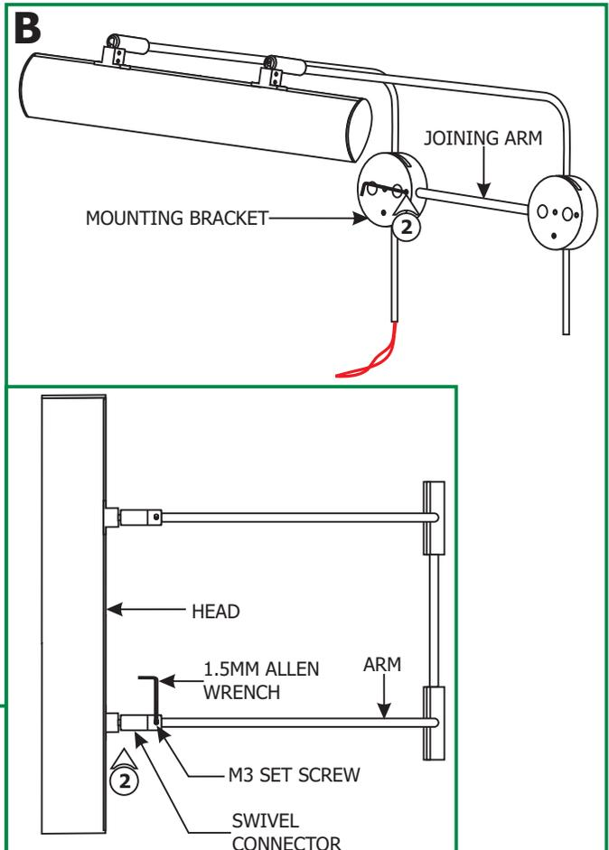
**2:** Insert the loose arm assembly (provided in the box) into the other swivel connector, insert the joining arm into the mounting bracket of the first arm. Tighten the M3 set screw on the swivel connector and mounting bracket with the 1.5mm Allen wrench.
