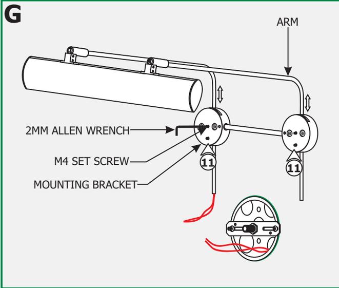
**11:** To adjust the height, loosen the four M4 set screw on the mounting brackets with the provided 2mm Allen wrench. Adjust the Cody to the desired height by sliding it up or down. Tighten the four M4 set screws with the 2mm Allen wrench.
