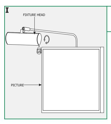
**15:** Rotate the fixture head to properly wash the picture with light.
