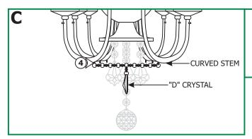
**4:** Install the six pieces of crystal marked "D" into the hoops located on the bottom of each curved socket stem, so that one end is hooked into one socket stem hoop and the other end into the adjacent socket stem hoop. Each curved socket stem will hold two crystal key rings when all crystals are installed.
