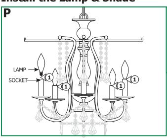
**CAUTION:** To reduce risk of a burn or electrical shock during lamping, disconnect the power to the fixture.
