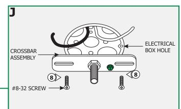
**8:** Mount the crossbar assembly to the electrical box holes with the two provided #8-32 screws
