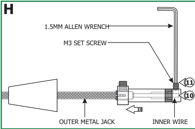
**10:** Keep feeding the coaxial cable in until the inner wire is visible in the screw hole of the fixture connector tip.
