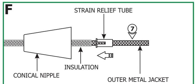
**7:** Feed the coaxial cable through the conical nipple and flared side of the strain relief tube. Slide the conical nipple down the coaxial cable. Slide the strain relief tube against the insulation.
