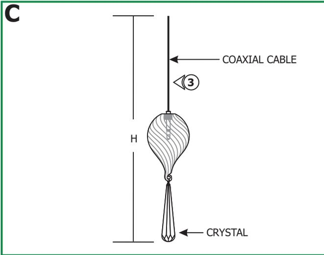
**3:** Cut the coaxial cable to the desired length (H) with a sharp cutter. The overall fixture height is measured from the bottom of the glass shade to the end of the coaxial cable.
