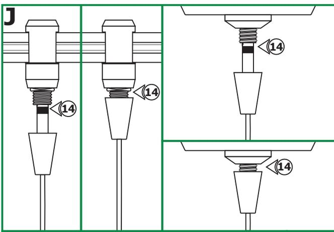
**14:** Use fingers to tighten the Fast Jack fixture connector into the Fast Jack system connector (Monorail, Monorail 2 Circuit, or canopy connector - Refer to the instructions provided with the system connector or canopy).
