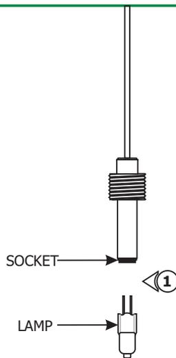
**CAUTION:** To reduce risk of a burn or electrical shock during lamping, disconnect the power to the fixture.
