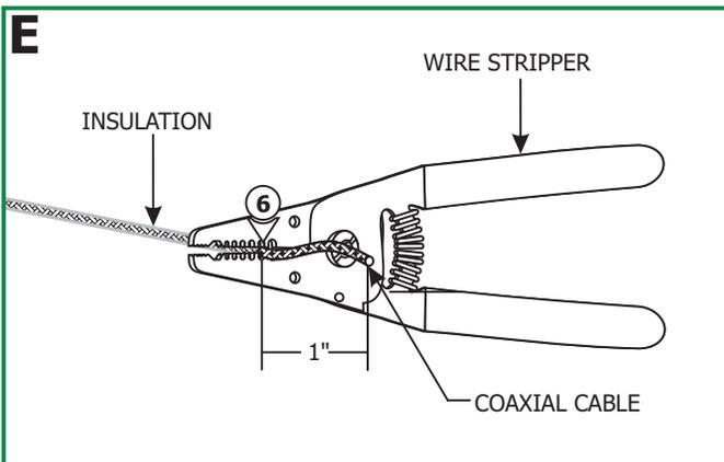
**6:** Use the #12 gauge hole of the AWG wire strippers to strip 1" of the insulation cover from the end so that the bare coaxial cable is exposed.
