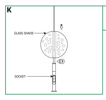
3: Carefully lower the glass shade onto the socket assembly.
