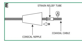
**4:** Feed the coaxial cable through the conical nipple and flared side of the strain relief tube. Slide the conical nipple and strain relief tube down the coaxial cable.
