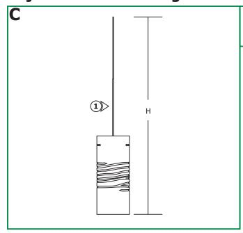
**1:** Cut the coaxial cable to the desired height (H) with a sharp cutter. The overall fixture height is measured from the bottom of the glass shade to the end of the coaxial cable.
