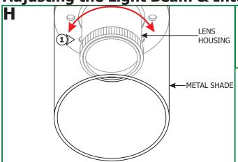
**1:** Rotate the lens housing (inside the fixture body) and set the beam spread to either spot or flood.
