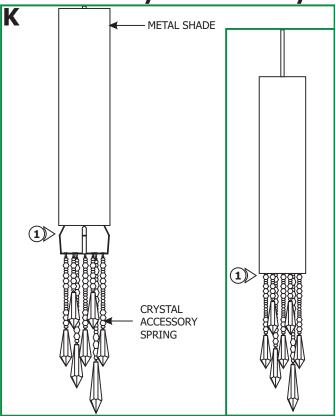
**NOTE:** Make all necessary adjustment to fixture, before crystal accessory (sold separately) is installed.
