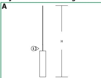
1: Cut the coaxial cable to the desired height (H) with a sharp cutter. The overall fixture height is measured from the bottom of the metal shade to the end of the coaxial cable.
