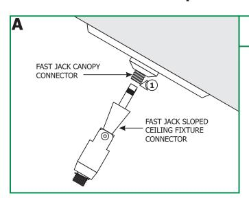
**1:** Use fingers to tighten the Fast Jack sloped ceiling fixture connector into the Fast Jack canopy connector.
