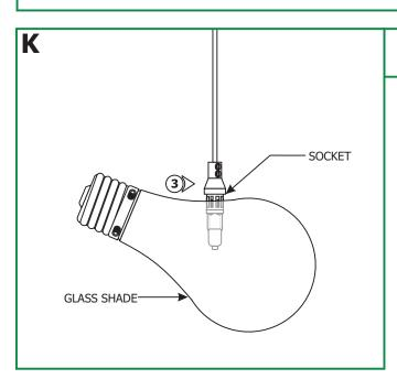
Use MAX 20 Watt, Type Bi-Pin Halogen Lamp.
