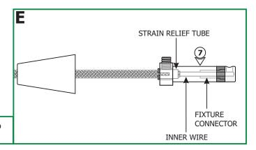
**7:** Feed the inner coaxial cable along with strain relief tube into the coaxial fixture connector.
