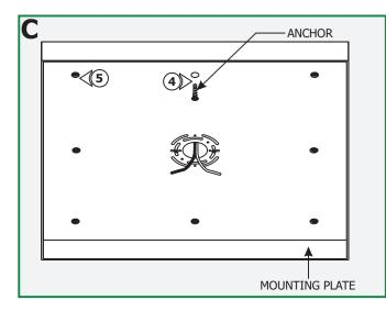
**4:** Tap the anchors through the mounting plate holes onto the marked point up to the threaded portion with a hammer.
