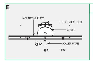
**7:** Slide the cover and mounting plate center hole onto the crossbar threaded nipple and secure it with the nut provided.
