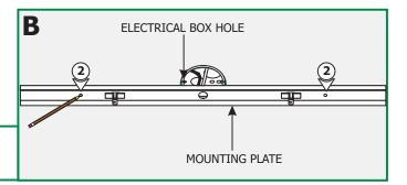
**2:** Align the mounting plate holes with the electrical box holes and mark a point through the mounting plate holes onto the ceiling. These points are used for the anchors.
