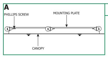
**1:** Loosen and remove the six Phillips screws from the canopy to remove the mounting plate.
