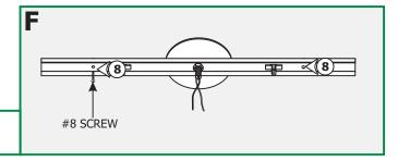
**8:** Secure the mounting plate to the anchors with the provided #8 screws.
