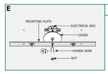
**7:** Slide the cover and mounting plate center hole onto the crossbar threaded nipple and secure it with the nut provided.
