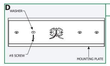
**6:** Secure the mounting plate to the anchors with the provided #8 screws and washers.
