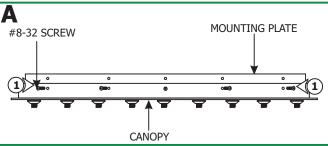
1: Remove the fourteen #8-32 screws around the canopy to remove the mounting plate.
