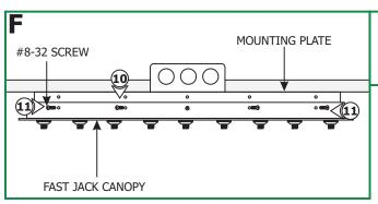
**10:** Place all wires and wire nut connections inside the canopy.
