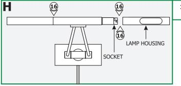
**16:** Pull out the two lamp housings from the fixture to expose the two sockets.
