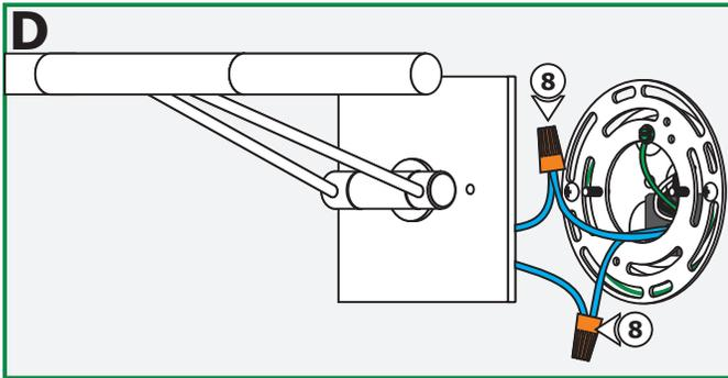
**8:** Connect each transformer low voltage (blue wire) to one fixture wire with a wire nut.
