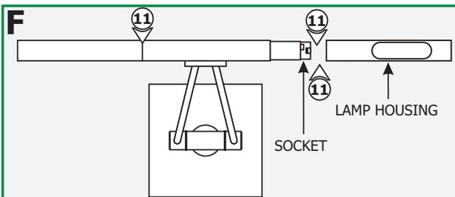
**11:** Pull out the two lamp housings from the fixture to expose the two sockets.
