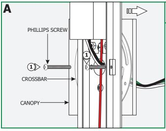
**1:** Loosen and remove the two Phillips screws in the center of the fixture to remove the crossbar.
