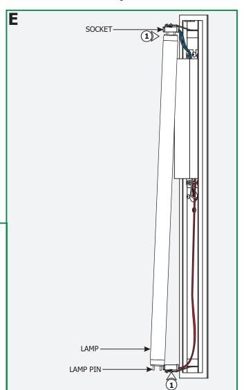
**<u>CAUTION:</u>** To reduce risk of a burn or electrical shock during lamping, disconnect the power to the fixture.
