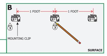
3: Place the mounting clips on the surface every 1' (measure from the the center of the mounting clip) and mark the screw locations.
