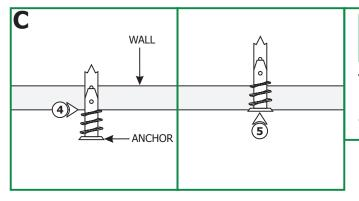
**NOTE:** Steps 4 and 5 are for drywall mounting. Omit these steps if mounting the clips to a wood surface directly. ANCHORS ARE NOT PROVIDED.
