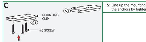
**5:** Line up the mounting clips to the anchors and secure it to the anchors by tightening the three #6 screws to each clip.
